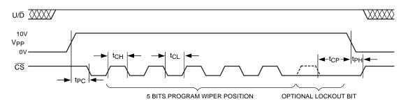
Figure 3. One Time Program Mode Serial Interface Timing Diagram
